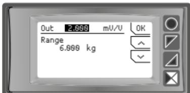
Use the arrow keys to set the correct mV/V ratio of strain gauge. Press “Ok” to confirm.
