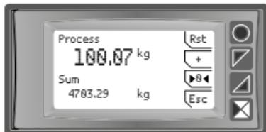
Press "Sum function" to enter the related page. Pressing "+" the **Process** value is added to the counter. It is possible to reset the total value keeping pressed "Rst" and to fix **zero** of the process pressing ">0<".
