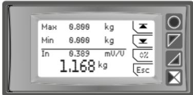
Press “” to calibrate lower limit and “” to for the upper limit. Press “%” to go back to calibration percentage.
