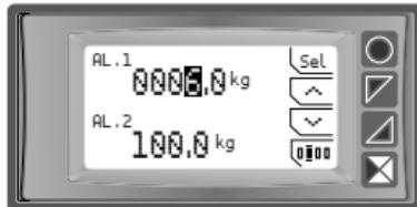
Press "Load data" to enter the thresholds modification.
