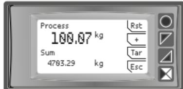
Press "**Sum Function**" to enter the function page. Pressing "+" the **Process** value is added to the counter. It is possible to reset the total value keeping pressed "Rst" and to fix "**tare zero**" of the process pressing "**Tar**".
