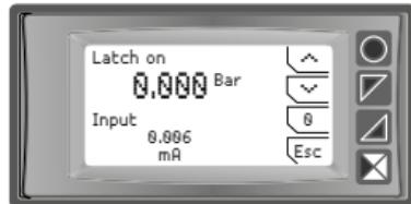
To use the LATCH ON function: enter configuration, select **Setting** on par. 8 **Latch on** and press "Sel" (STR551 shows the page in the picture).
