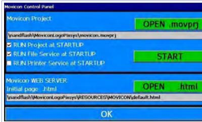
Use this window to select the services and programs relating to Movicon 11 to be run automatically when starting the device.
