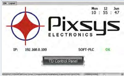
When starting the device, a project opens that allows you to verify the general status of the machine, system date and time, associated IP address, SoftPLC running in the background.
