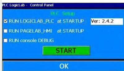
Use this window to enable/disable the running of the SoftPLC when starting the device. When you select the “RUN console DEBUG” flag while running the SoftPLC, the Debug window will be compiled with the system events in real time to be able to check any anomalies.
