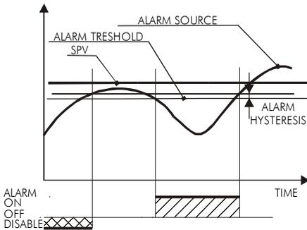
This alarm is disabled at the starting of PL300 and it is automatically activated when the alarm source exceeds the alarm threshold of a value which is equal to the hysteresis. Then the alarm works like the above described “deviation low alarm”.
