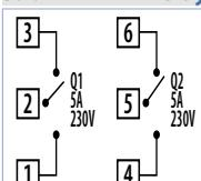
Capacity 5 A / 250 VAC for resistive loads.
