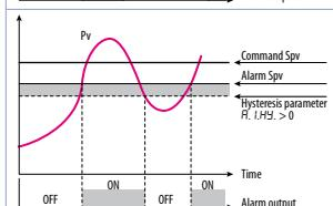
Upper deviation alarm value of alarm setpoint less than "0" and hysteresis value greater than "0" (Par.128  $R.I.H$  > 0).
