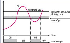
Lower deviation alarm value of alarm setpoint greater than "0" and hysteresis value greater than "0" (Par.128 R.I.HS > 0).
