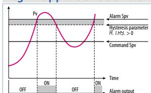
Upper deviation alarm value of alarm setpoint greater than "0" and hysteresis value greater than "0" (Par.128  $R.I.H$  > 0).
