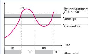
Lower deviation alarm value of alarm setpoint less than "0" and hysteresis value greater than "0" (Par.128 R.I.HS > 0).
