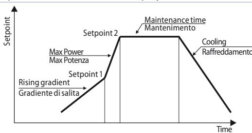
Cycle starts at each activation of the controller, or via digital input if it is enabled for this type of functioning (parameters 231, 239 set as *St./St.* or *RuN*).
