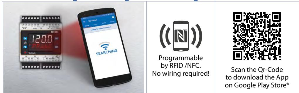
The controller DRR244 is supported by the App MyPixsys: using an ANDROID smartphone with NFC connection it is possible to program the device without using a dedicated equipment. The App allows to read, set and backup all parameters which are stored into the internal memory of Pixsys devices.
