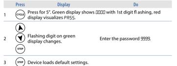
Entering password 9999 all default parameters will be loaded. If it is necessary to cancel and reset also the cycles, enter password 9989.
