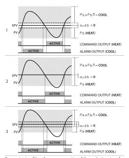
Parameter E.c.? has the same meaning of the cycle time E.c. for heating.
